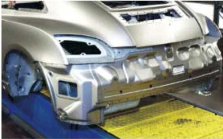
**Figure 1 – A spot-welded vehicle body-in-white [1].**
